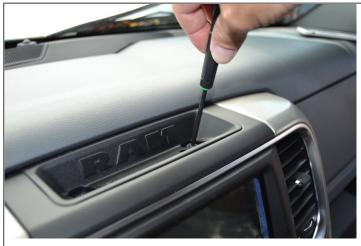
2. Remove the two screws from the bottom of the pocket. A Torx head screw driver might be needed for the screws being removed.
