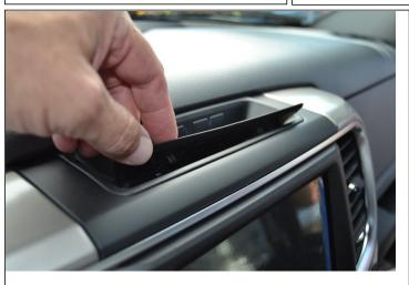
1. Remove the rubber pad at the bottom of the shallow pocket in the top center of the dash.
