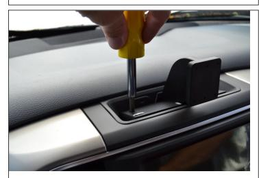
3. Align the holes in the bottom of the ProClip with the threaded holes where you removed the dash screws. Insert the included screws through the holes in the bottom of the ProClip mount and secure the mount by tightening the screws into the threaded holes in the bottom of the dash pocket.
